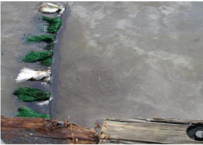
Figure 4.2 Oil sticks to pom poms on a rope (USCG, 2008).
