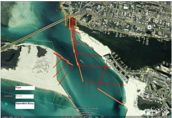
Figure 5.1 Boom Deployment Configuration in East Pass
