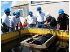
Figure 3.3 Oleophilic drum skimmer (Offshore Technology, 2003).
